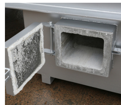
Ash Door View
