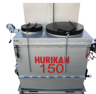
Circular Loading Hatches: Ideal for Bagged Medical Waste
