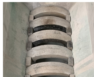
The unique hearth bar technology allows for efficient incineration from above and below.
