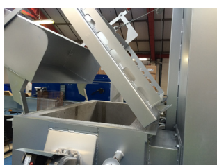
Semi-automatic loading hopper for controlled loading and operator safety.
